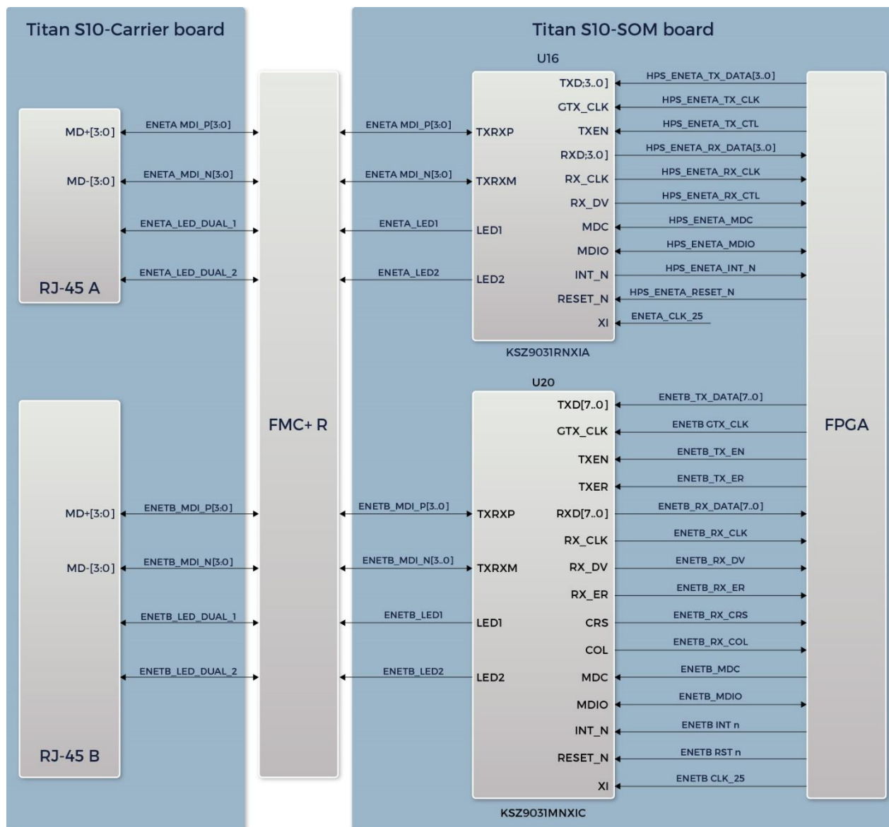
Figure 2-13 Connection between the RJ45 connectors and Stratix 10 FPGA
