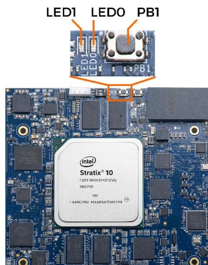
Figure 2-6 Position of all the user LEDs/Switches/Buttons
