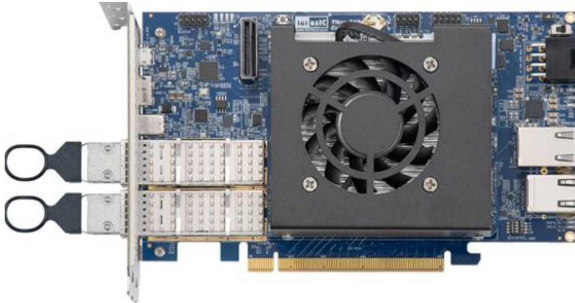
Figure 8-2 QSFP Transceiver Loopback Test in Progress
