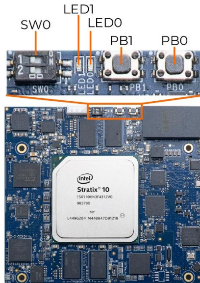
Figure 2-8 Location of the KEY and LED on the kit
