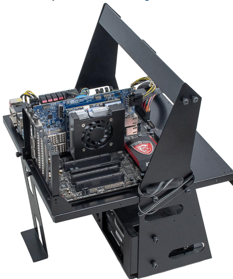
Figure 5-9 FPGA board installation on PC
