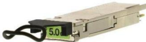
Figure 8-1 QSPF Loopback Fixture
