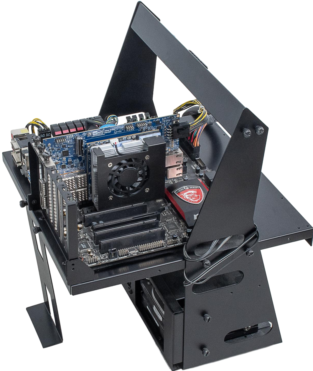
Figure 6-4 FPGA board installation on PC
