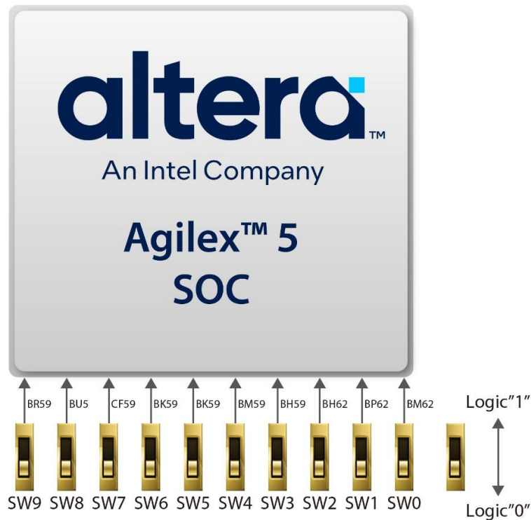
Figure 3-20 Connections between the slide switches and the Agilex 5 SoC FPGA
