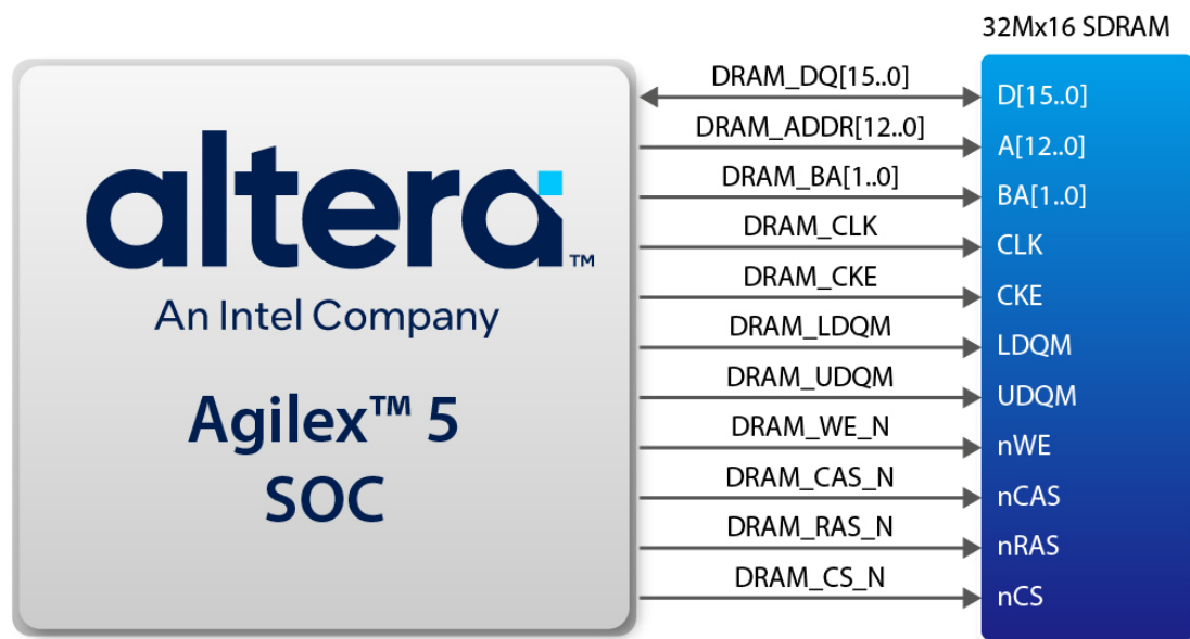
Figure 3-31 Connections between the FPGA and SDRAM
