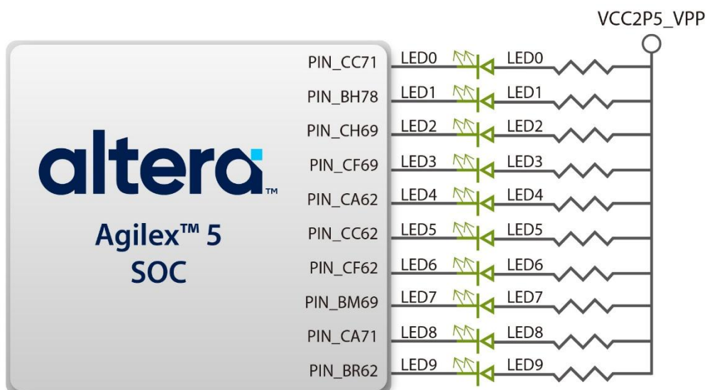
Figure 3-21 Connections between the LEDs and the Agilex 5 SoC FPGA
