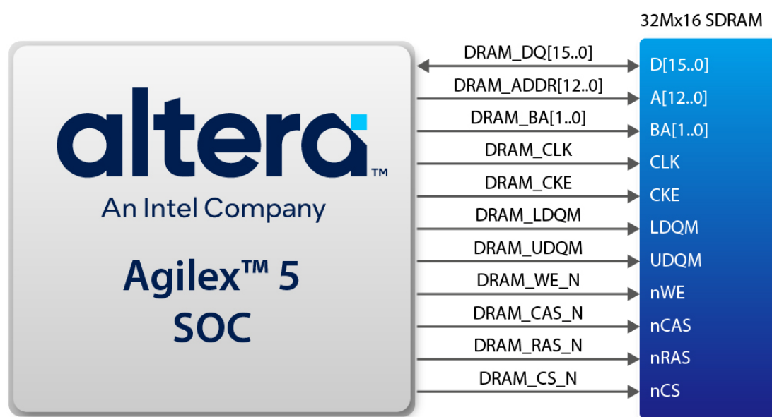
Figure 3-31 Connections between the FPGA and SDRAM
