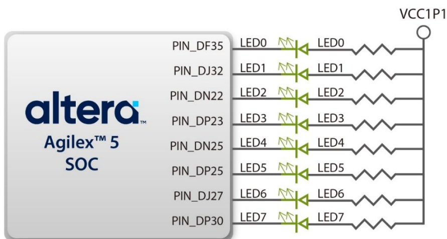
Figure 3-17 Connections between the LEDs and the Agilex 5 SoC FPGA
