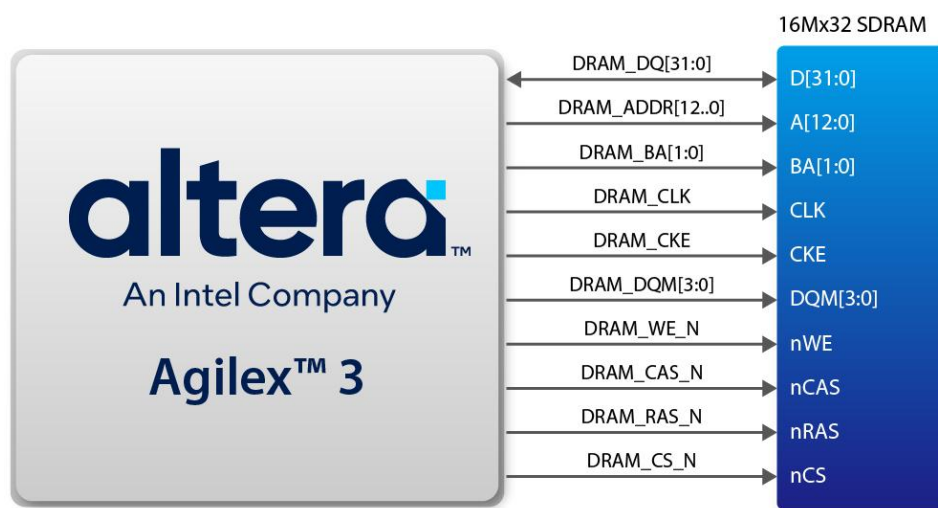
Figure 3-19 Connections between the FPGA and SDRAM
