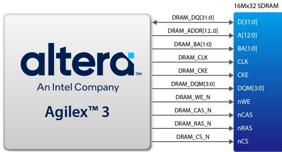
Figure 3-19 Connections between the FPGA and SDRAM
