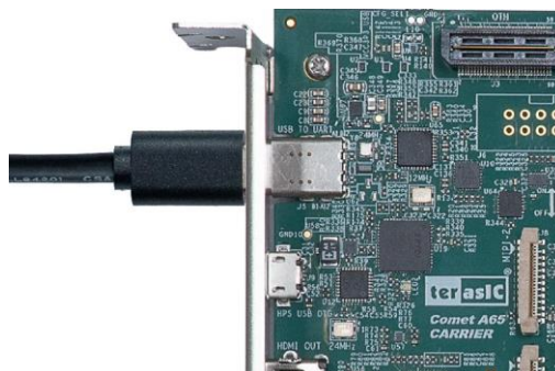
Figure 3-2 Connect USB type-C cable to the board
