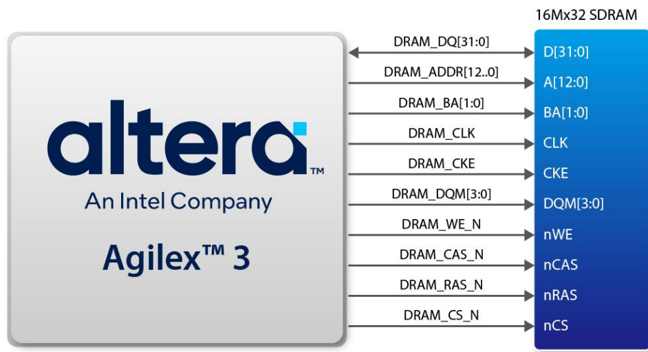
Figure 3-19 Connections between the FPGA and SDRAM
