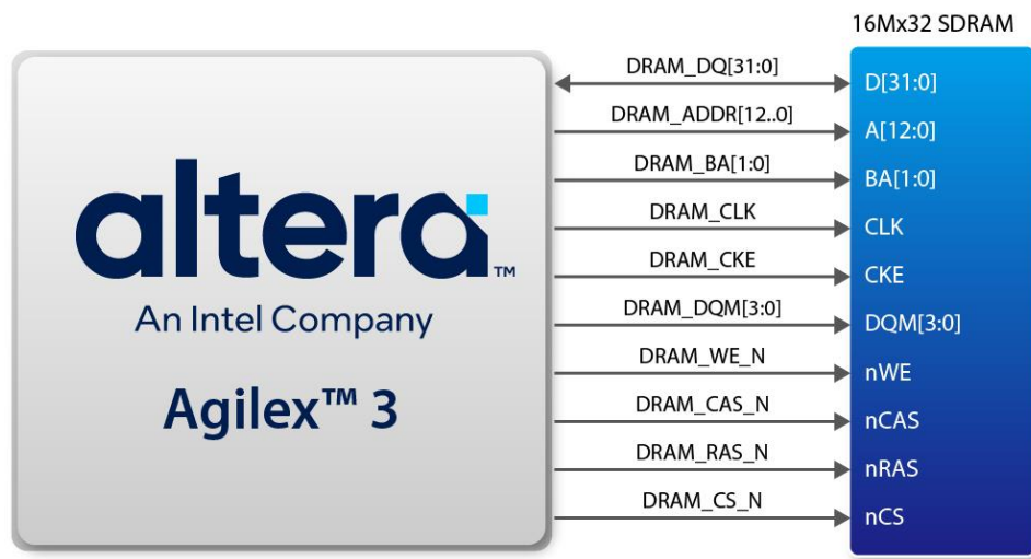
Figure 3-19 Connections between the FPGA and SDRAM
