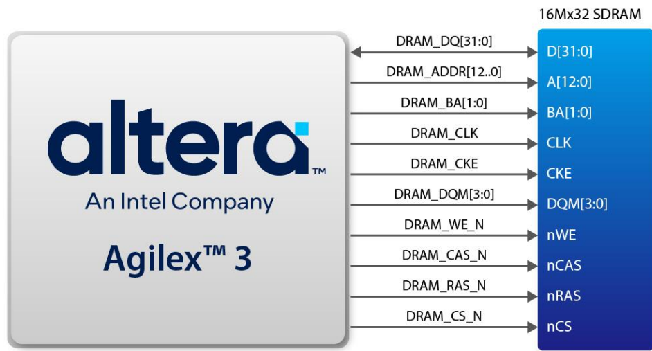
Figure 3-19 Connections between the FPGA and SDRAM
